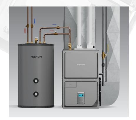
The NPF System Furnace is an integrated combination of the NPF Hydro-furnace and an indirect tank. The NPF's unique forced-air technology heats air using water. The NPF system furnace is different from the standard NPF furnace in that it can also use that heated water to heat the water in a stainless steel indirect storage tank. That heated water can then be used for domestic hot water or utilized in a hydronic zoned heating system.
